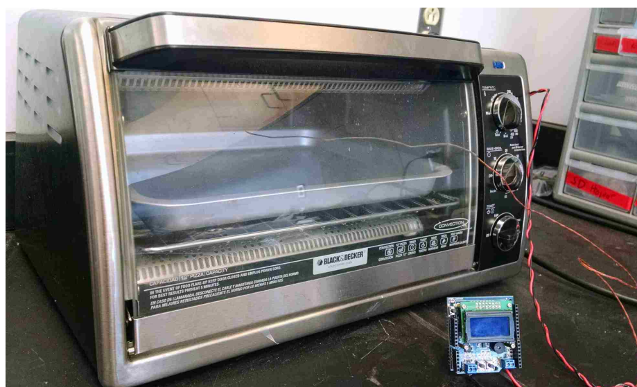
Figure 2.10: Surface mount soldering reflow oven made from a standard toaster oven. In order to achieve a high enough temperature to properly solder the components, a toaster oven was chosen that could reach 500 degrees Fahrenheit.
